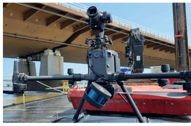
With Hovermap mounted beneath the drone and a high resolution RGB camera on top, GeoZICHT captured sharp and actionable inspection data of the complete bridge.
