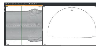
The Hovermap point cloud in .laz can be imported into 3D software to quickly and easily calculate measurements and volumes for the scan.
