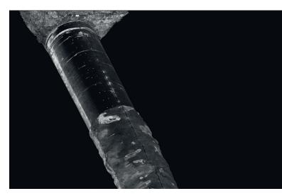
The LiDAR scan provides Brierley Associates with highly detailed baseline data that will allow them to monitor thousands of points within the tunnel for change and detect issues and potential points of failure faster.
