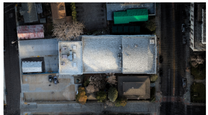
Overhead external view of the Center for the Arts. This colorized point cloud data, captured by Hovermap in a 15-minute drone flight, provides accurate dimensions of the venue surrounds and enables better management of the external space during events.
