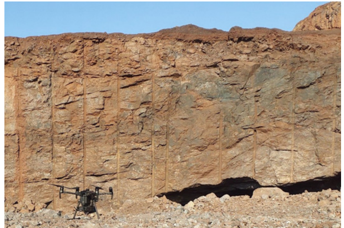
Hovermap at the entrance of the pit void that DMS scanned in a 5-minute beyond-line-of-sight flight.
