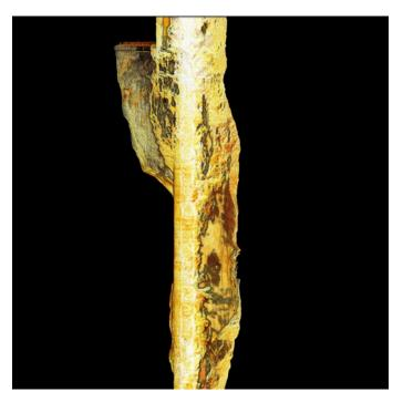
Hovermap reduces these risks by removing personnel from hazardous areas and minimizing the time taken to map inaccessible vertical voids. When drone-mounted, Hovermap enables autonomous flight and collision avoidance capability to produce shadowless, high resolution scans of underground voids. Or it can be attached to a tether and lowered into voids too narrow to fly. Mining or geotechnical engineers can quickly and safely inspect orepasses, raises or vents with minimal disruption to production.
