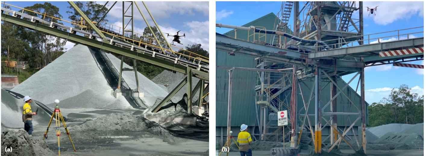
Figure 2 Hovermap as mounted to the DJI M210 deployed across the study area in (a, b) two flights and a walking scan of a crushing plant.
