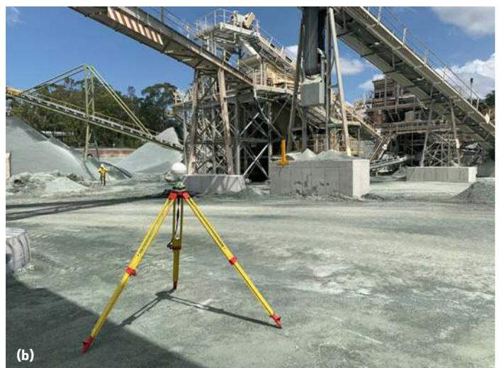
**Figure 1** Establishment of control across the study area using four prisms that were (a) located with a total station. Prisms were replaced with (b) spherical targets with the same vertical offsets during the Hovermap scanning.
