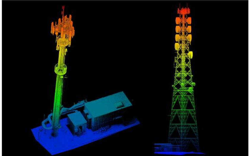
Hovermap's advanced collision avoidance and autonomy capabilities keep the drone at a safe standoff distance, reducing risk to the asset. These point cloud data sets were captured within a single flight and colored by elevation. Additional cameras can be carried for condition assessment.
