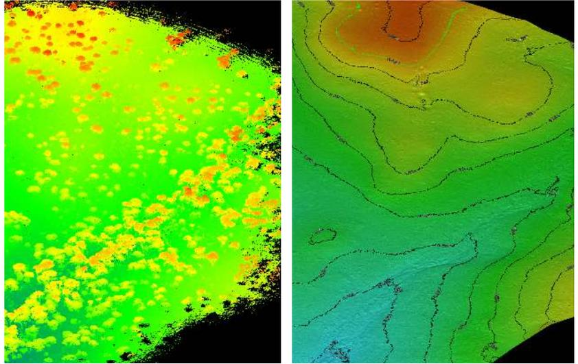
Captured with Hovermap (left), vegetation has been removed to produce a DTM (right) of the study area.
