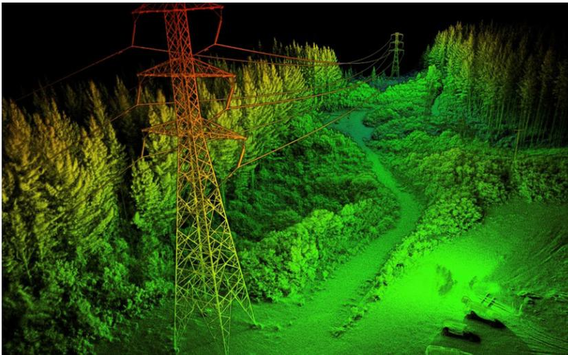
Hovermap's collision avoidance and virtual shield ensure the drone maintains the standoff distance from these critical structures.
