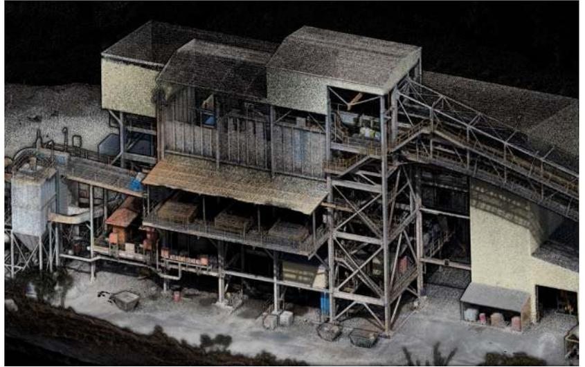
Previous inspections at this site were hampered by the metal structures interfering with drones' magnetometers. Hovermap uses only LiDAR data so is unaffected by potential interference from large metallic structures and GPS shadows.
